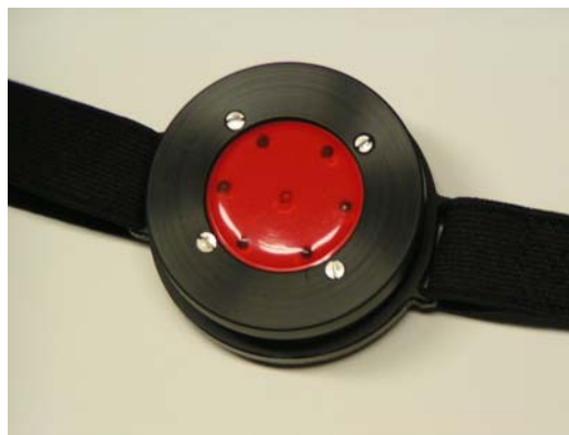
Fig.6. External view of the developed photoplethysmograph
