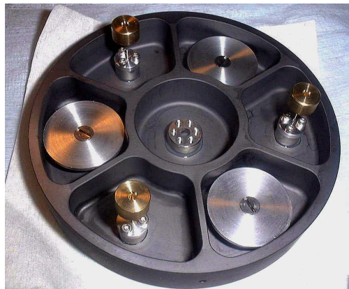
Fig. 3: Back side of SiC mirror for NAOS Field Selector
