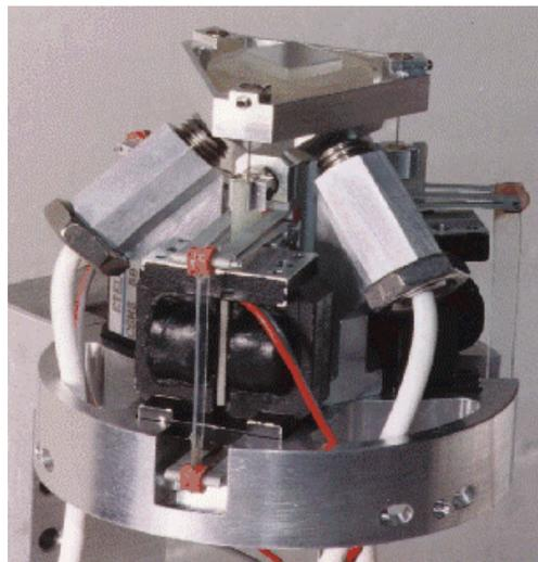
**Fig. 8:** Photograph of two-axis tilt fine-pointing assembly prototype
