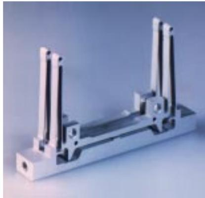
**Fig. 2:** A monolithic "hairpin" compensated parallelogram. The size of the baseline model is about 4 cm and its motion range is  $\pm 1$  mm but the concept is scalable both to smaller and large dimensions.
