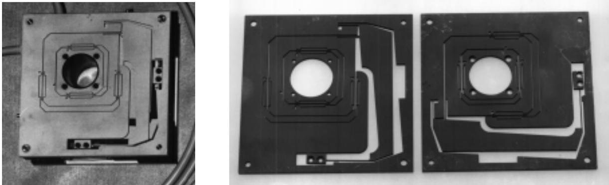
**Fig. 1:** Micropositioning stage for an optical fiber system. The mechanism is constituted by two monolithic components (each one machined for a single plate such that it forms a system of multiple levers linked by flexure blades) which provide the guiding and reduction of the motion, as well as a complete uncoupling between the two main directions.
