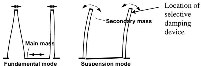
**Fig. 3:** The fundamental mode and of one of the main disturbing modes.
