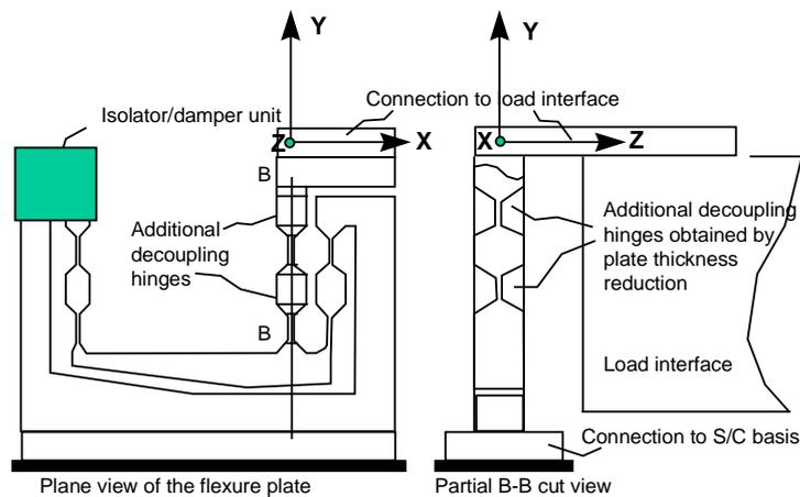
**Fig. 5:** Basic concept for a single-degree-of-freedom isolation/damping element
