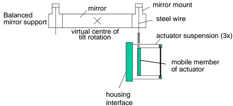
**Fig. 7:** Principle of 2-axes mirror suspension
