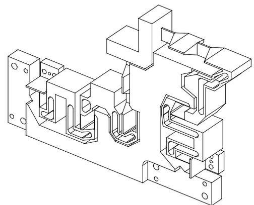
**Fig. 6:** 2-DoF Mechanical Element for Damping and Isolation (MEDI). Right, a drawing of the rather complex monolithic flexure structure which provides both the uncoupling and the amplification functions of the MEDI.
