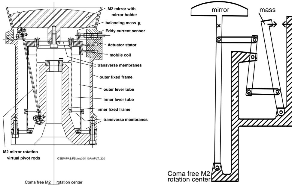
**Fig. 10:** Basic flexure kinematics of the coma-free secondary mirror unit: note that the rotation point is far outside the envelope of the system. Right, the corresponding kinematic theoretical mechanism, which if based on stiff members and hinges would require a much large volume
