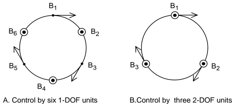
**Fig. 4:** Two possible configurations for 6-DoF load position definition
