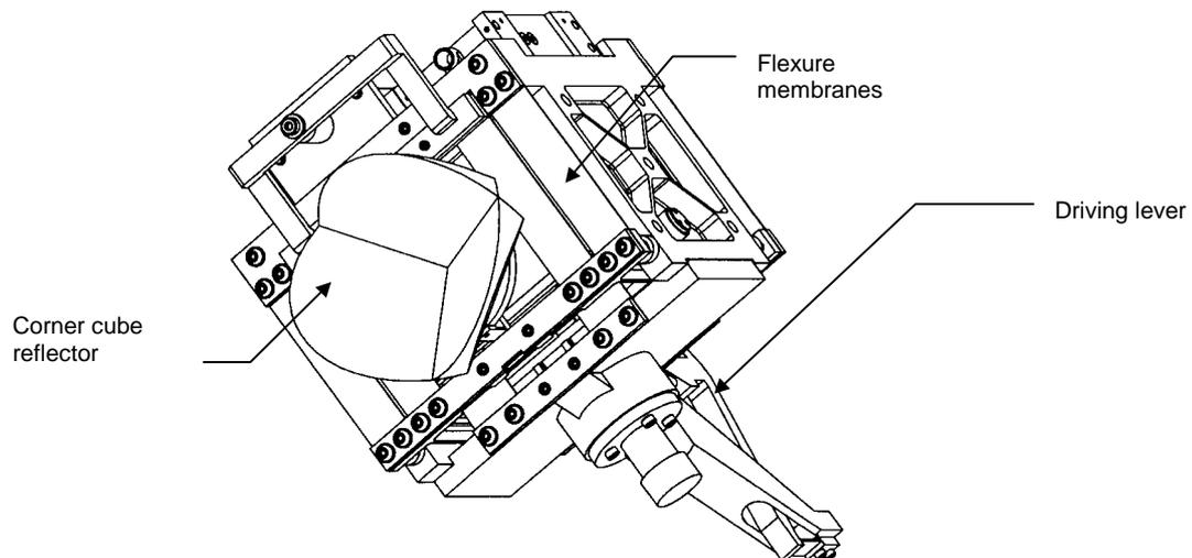
**Fig. 11:** IASI Corner Cube Mechanism
