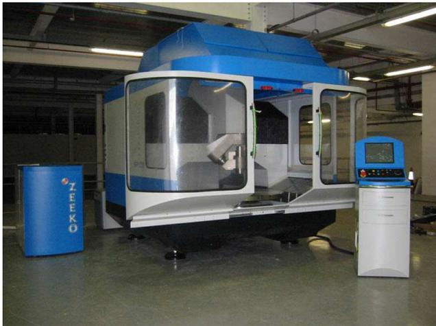
**Fig. 8** Zeeko 1200mm CNC Classic/Fluid-jet polishing machine.
