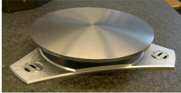
Figure 8: The curved steel focal plate.
