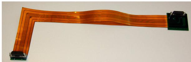
Figure 7: The flexible printed circuit used in StarPicker.
