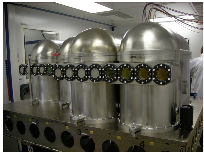
Figure 9, left: CAD of the DDL system infrastructure showing the tables, the vacuum vessels and the front-end electronic box. Right: Picture of the actual system during integration in Europe.
