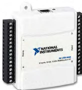
FIGURE 37 – Interface LabView NI USB-6008.
